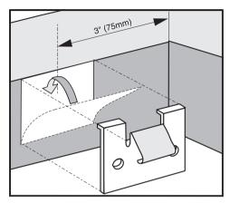
■ For granite countertops, the spring clips must be placed in position and secured with strong, double-sided adhesive tape.
